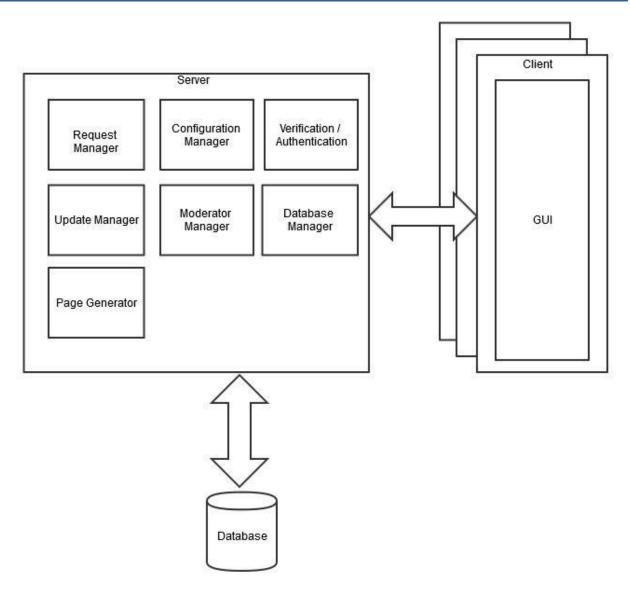
The server communicates with the database to get user data (such as account details and settings) and other necessary data. This data, along with other data (possibly from other databases) is used to generate a page. The pages will likely be generated using php. The server is also responsible for authenticating the user. The client will communicate to the server through a session.
